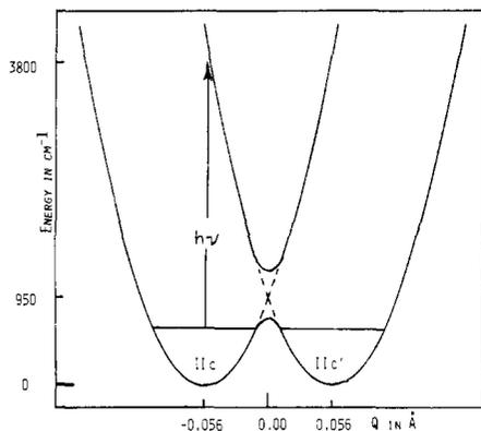
**Figure 2.** Potential surface and ground-state vibrational level for the interconversion of IIc and IIc'.  $Q$  = reaction coordinate =  $\sqrt{2}[R_{CO}(12) - 1.26 \text{ \AA}] = \sqrt{2}[1.26 \text{ \AA} - R_{CO}(9)]$ .
